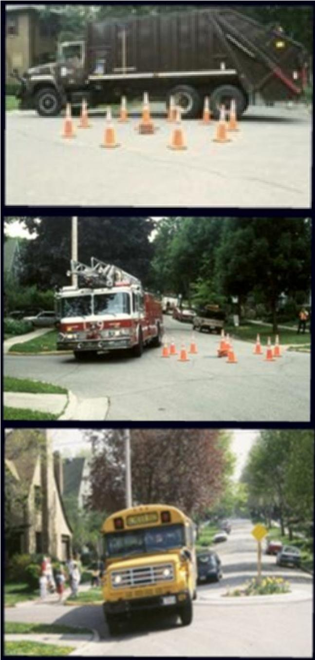
*Figure 11 testing of traffic circles for large vehicles*
